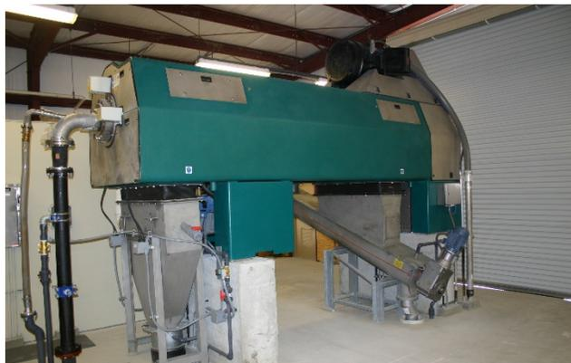
Picture #1: Centrifuge utilized to dewater the alum floc
