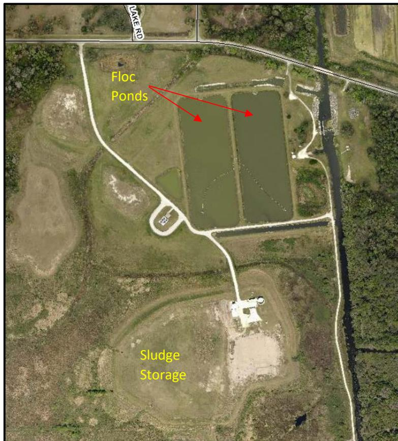
Figure 1. NuRF Layout showing the Two Floc Ponds and the Sludge Disposal Area.
